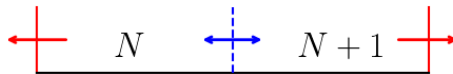
Figure 1: An illustration of the difference between two TMMC simulations with a single macrostate (top) and one TMMC simulation with double macrostates (bottom). In the GCE, the macrostates are the number of fluid particles, N . The arrows indicate trials which attempt to change the macrostate (i.e., insertions and deletions). The single red arrows indicate an attempt to change the macrostate outside the bounds of the simulation. The blue double arrow represents neighboring macrostates in a TMMC simulation which are in the allowed range, and thus trial attempts between these macrostates may be accepted.
